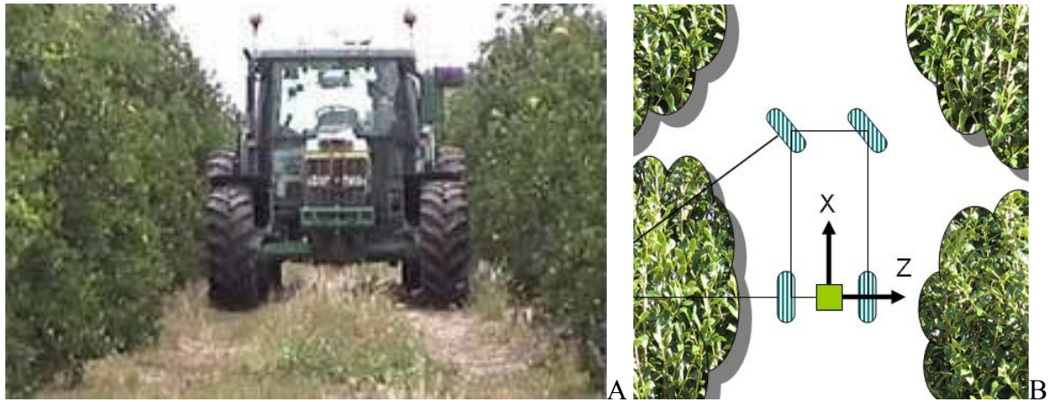
Figure 4-1. Vehicle system. A) Scouting autonomous vehicle (Subramanian, V., 2006). B) Motion model of vehicle.
