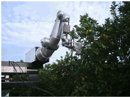
Figure 8-26. Outdoor experiment. A) Scanning using robot manipulator with B) zigzag camera motions.
