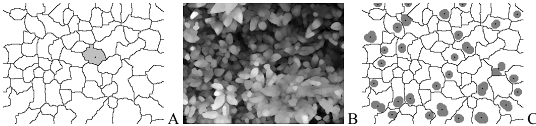
Figure 5-5. Detect the center of segment. A) Segmented patch. B) Image applied an opening with small mask. C) Detected feature points.
